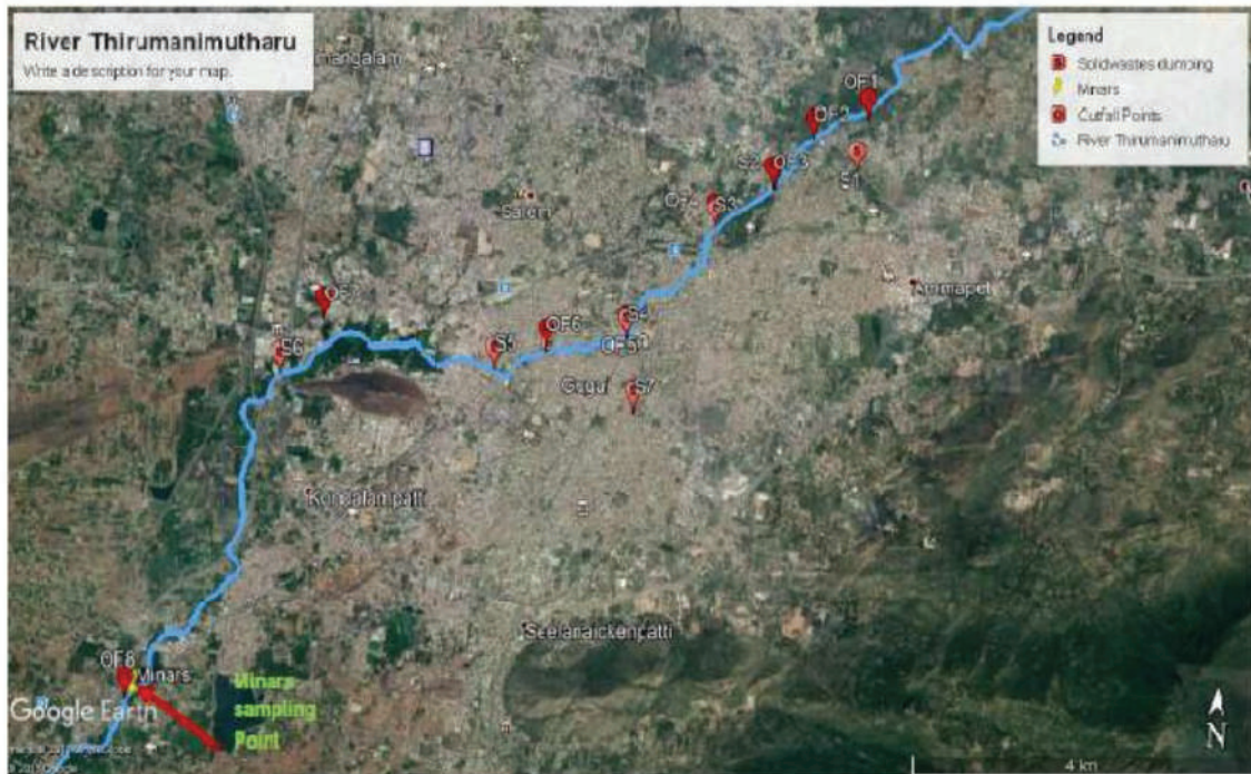
Figure 101: Sewerage outfall and solid waste dumping points along the river
